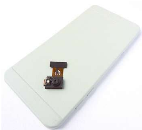
Figure 6: Example of a customer 3D TOF camera for mobile applications using the epc660 chip
