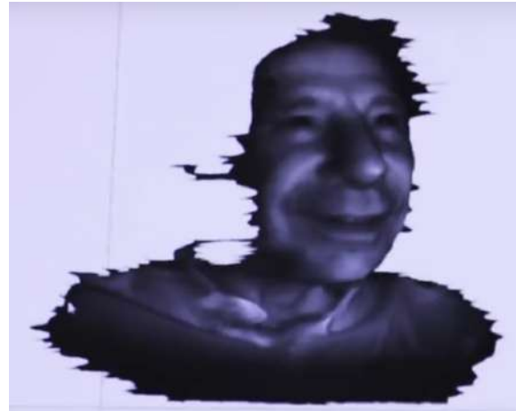
Figure 1: 3D facial scanning with epc660
