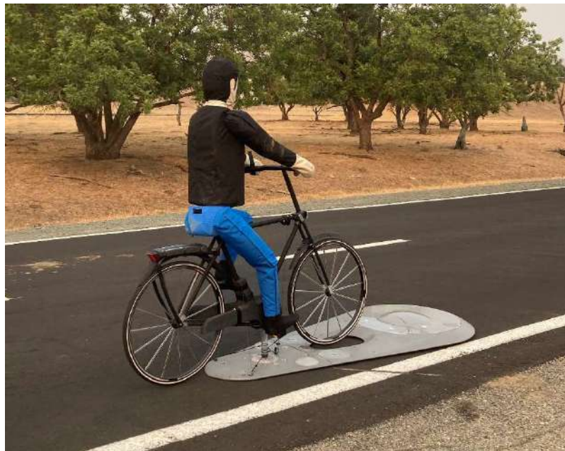
Figure 8: 4activeFBsmall platform with 4activeBS-adult cyclist target Image Source: AAA
